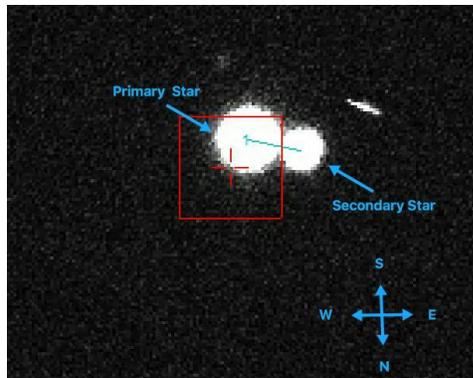
**Figure 3.** Mira Pro locating the centroids of the primary and secondary stars, dictated by the teal line, to perform astrometric measurements. The cross hairs centered on the red box are the coordinates of HJ 5439.
