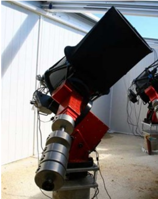
Figure 2. T7 17-inch Planewave f/6.8 Corrected Dall-Kirkham (CDK) Astrograph in Spain.
