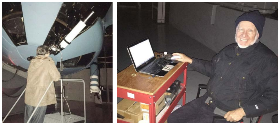
Figure 4. Left: Dave Rowe centers a double (binary) star using slow motion controls. Right: Russ Genet operates the EMCCD camera from a laptop using Andor's Solis software.
