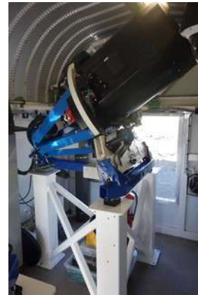
Figure 1: An LCO custom Meade 0.4-meter telescope with SBIG STX-6303 camera used to image the selected double stars. (Source: LCO)
