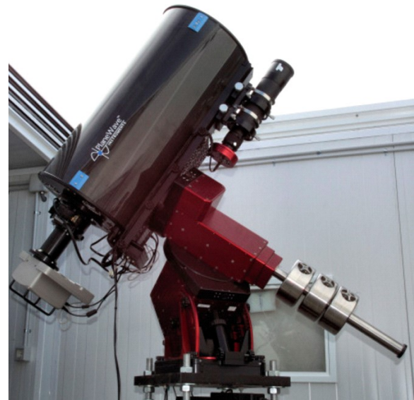
Figure 2. T18 Telescope based out of Nerpio, Spain. From the iTelescope Network. Telescope Specs: TEL 0.32-m f/8.0 reflector + CCD, Resolution: 0.73 arc-seconds/pixel, UTC +1:00 Madrid Daylight Savings Time is Observed, Minimum Target Elevation: Approximately 30^\circ - 40^\circ Degrees, North: 38^\circ 09' West: 002^\circ 19' , Elevation: 1650m
