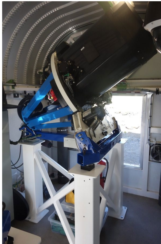
Figure 1: Image of the 0.4 meter telescope with the SBIG STL6303 cameras, provided by Las Cumbres Observatory
