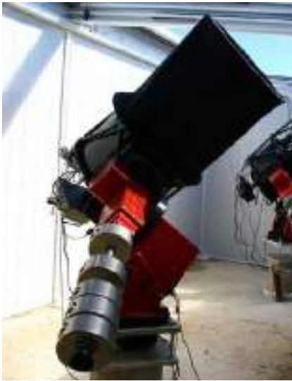
Figure 4. T7 17" PlaneWave f/6.8 CDK Astrograph with SBIG STL11000M CCD in Nerpio, Spain.
