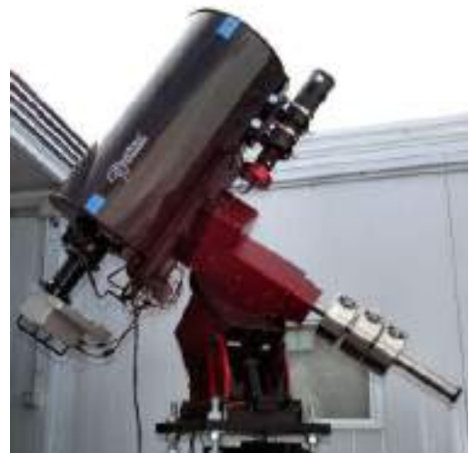
Figure 5. T18 12" PlaneWave f/7.9 CDK Astrograph with SBIG STXL-6303E CCD in Nerpio, Spain.
