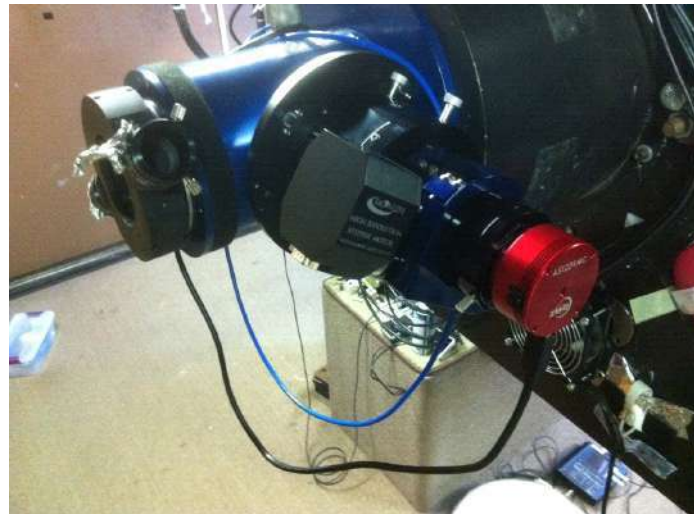
Figure 3. Close-up of the TAI 24-inch optical paths for Speckle Interferometry. A 30mm illuminated reticle eyepiece (not shown) was installed in the “open” path at left. For the engineering run, a ZWO ASI290MM speckle camera was used in place of the ZWO ASI224MC seen here.
