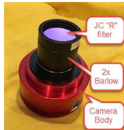
Figure 3. ZWO ASI290MM monochrome CMOS camera, 2x Barlow lens, and Johnson-Cousins "R" filter. (Image by Richard Harshaw).
