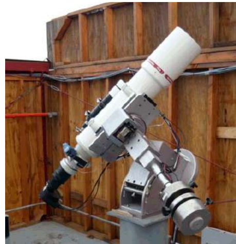
Figure 2. T3 in New Mexico Optical Design: Apochromatic Refractor Aperture: 150mm Focal Length: 1095mm F/Ratio: f/7.3 Mount: Paramount GTS Instrument Package CCD: SBIG ST-4000XCM One Shot Color CCD Resolution: 1.45 arc-secs/pixel Array: 2048 by 2048 (8.3 Mega pixels) FOV: 49.6 x 49.6 arc-mins Observatory: Mayhill, New Mexico
