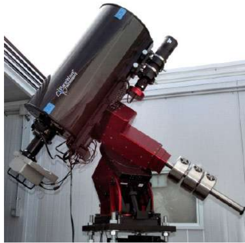
Figure 1. T18 in Spain . Optical Design: Corrected Dall-Kirkham Astrograph Aperture: 318mm Focal Length: 2541mm F/Ratio: f/7.9 Mount: Paramount PME Instrument Package CCD: SBIG STXL-6303E Non Anti-Blooming Gate (NABG) Resolution: 0.73 arc-secs/pixel Array: 3072 by 2048 (6.3 Mega pixels) FOV: 37.41 x 24.94 arc-mins Observatory: Nerpio, Spain
